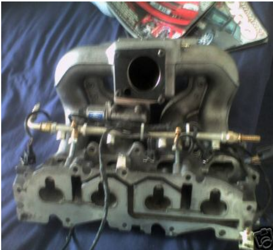
picture above is a 1.8 inlet with custom made injector rail
